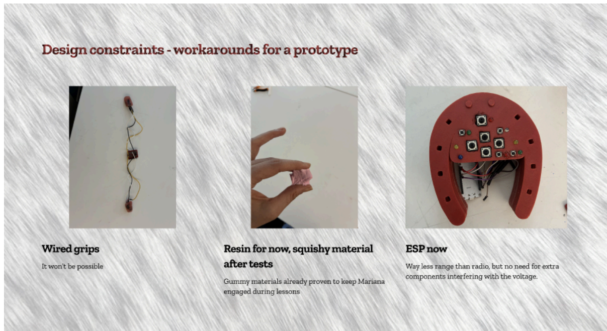
Figure 7. Design considerations and constraints — side-by-side comparison of initial design phase intentions (movable grip element, exploratory sensory materials, 433 MHz radio technology) versus final prototype decisions driven by real-world constraints (wired grips as interim solution, resin enclosure for now, squishy grip surface confirmed after tactile tests, ESP-NOW replacing radio after voltage mismatch).'
